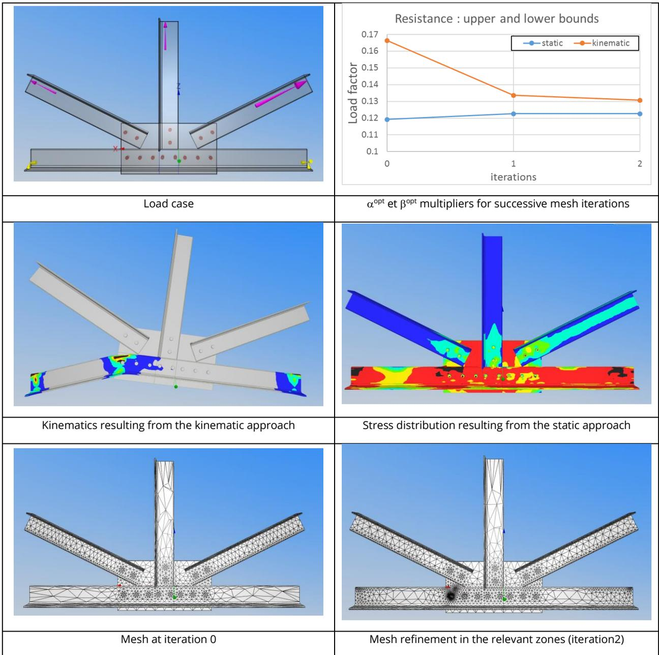
Figure 1. Re-meshing iterations and the convergence of static and kinematic results
