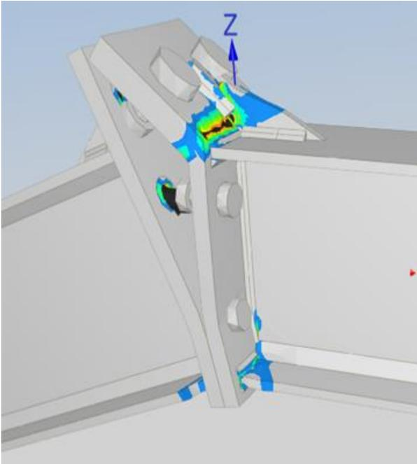
Figure 2: ULS plastic flow from kinematic approach on a simple beam-to-beam bolted connexion.
